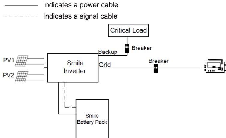
Off-Grid (with Generator) Storage System – Scheme
