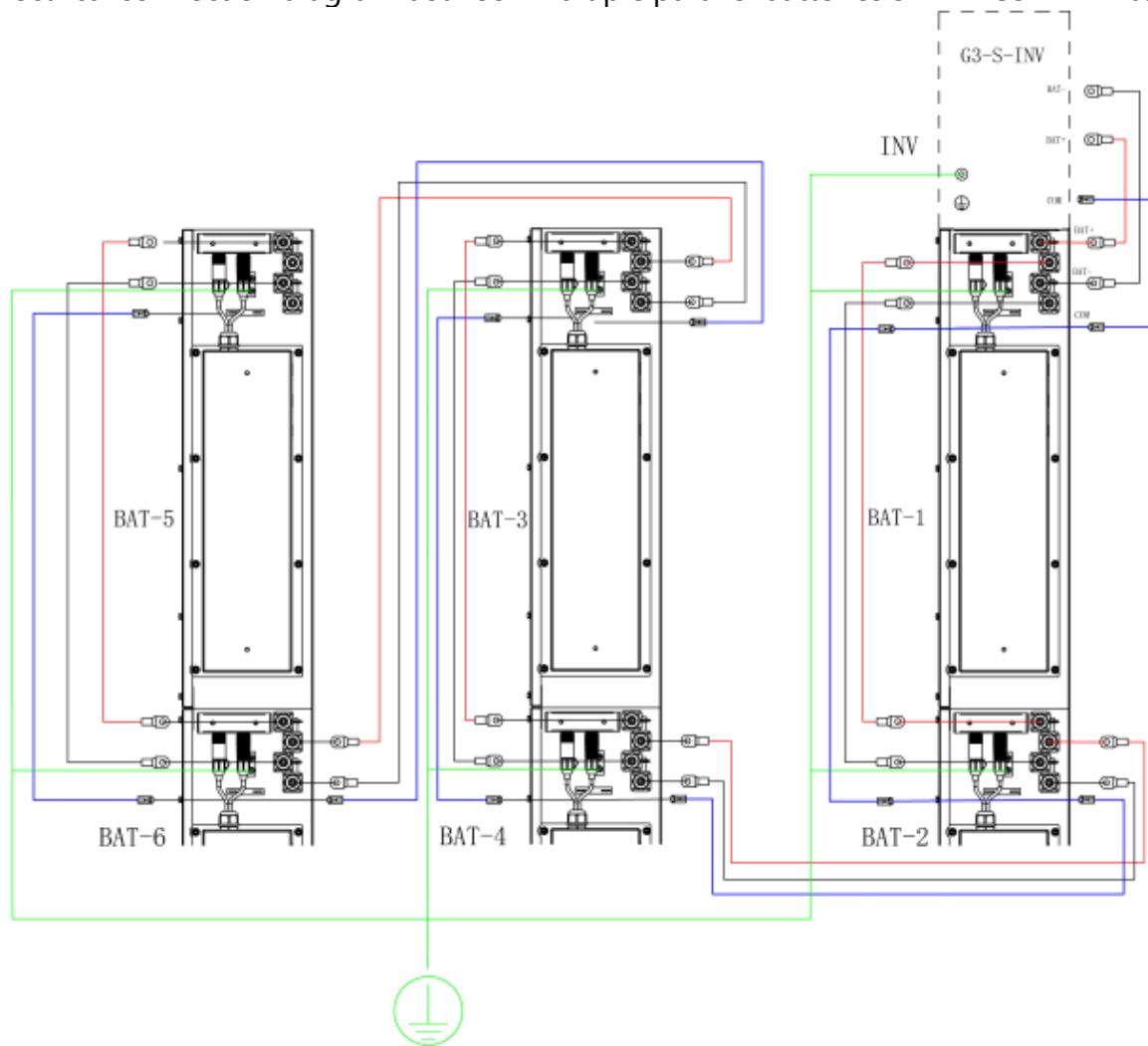
Remove the excess terminal resistor
