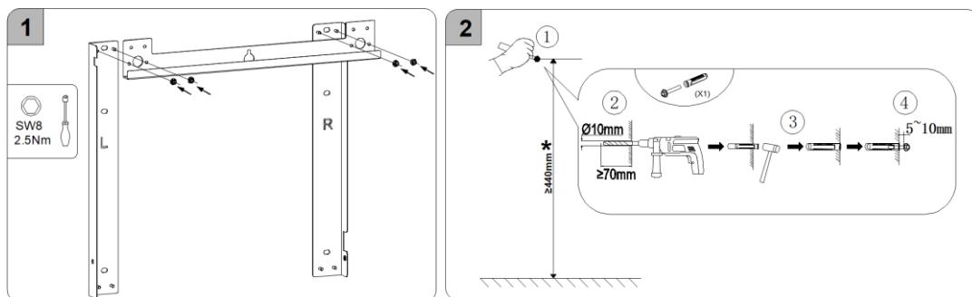
\*This recommended value "440mm" is for wall bracket location of the bottom battery. Depends on the number of expansion batteries mounted later, it is advisable to have a minimum of 150~200mm off the ground to protect from submergence.
