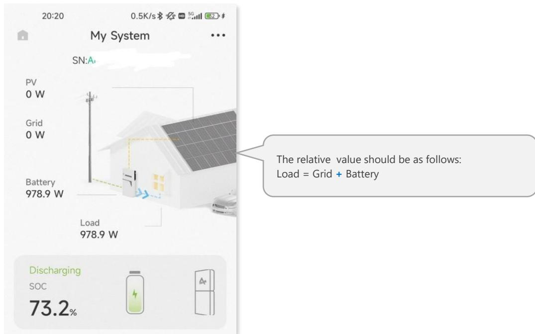
**Step 2:** Please switch on the PV switch on the energy storage inverter and the AC breaker on the PV inverter if there is any. Check the running status of the system.
