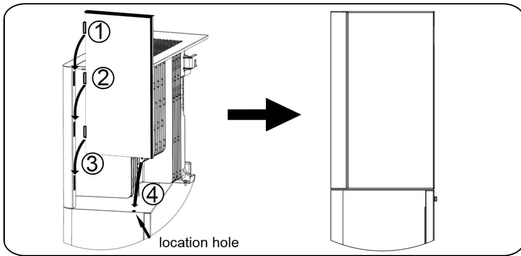
c. Cut a cable hole based on the AC cabling routing, and route the cables through the cable hole. Align the hooks on the side of the cable cover with the slots on the front cover side, secure the cable cover to the inverter (tool: T20 screwdriver, torque: 1.6Nm)
