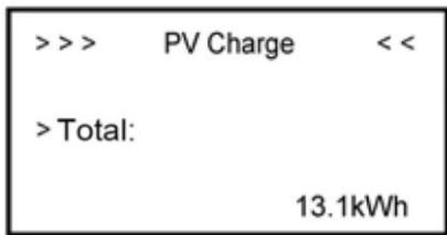
PV Charge interface displays total battery energy charging from the PV-panels.
