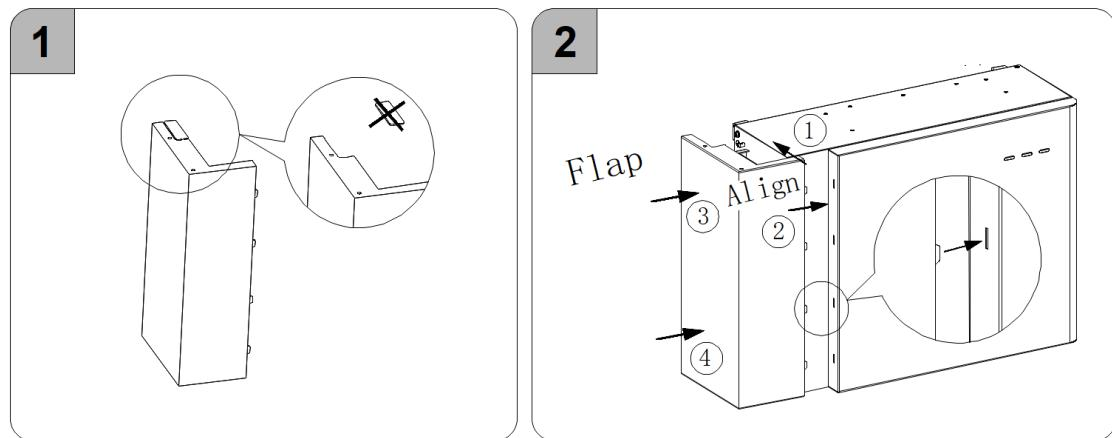
Disassemble the cable cover of the battery SMILE-G3-BAT-4.0S
