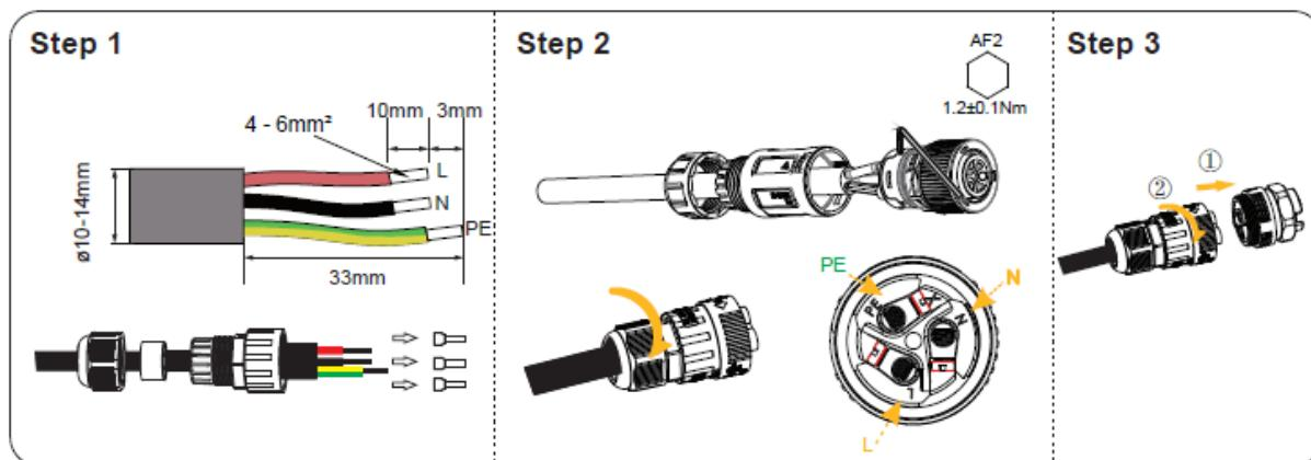
The above wiring steps are only suitable for backup connection of SMILE-G3-S5/S3.6/B5-INV.
