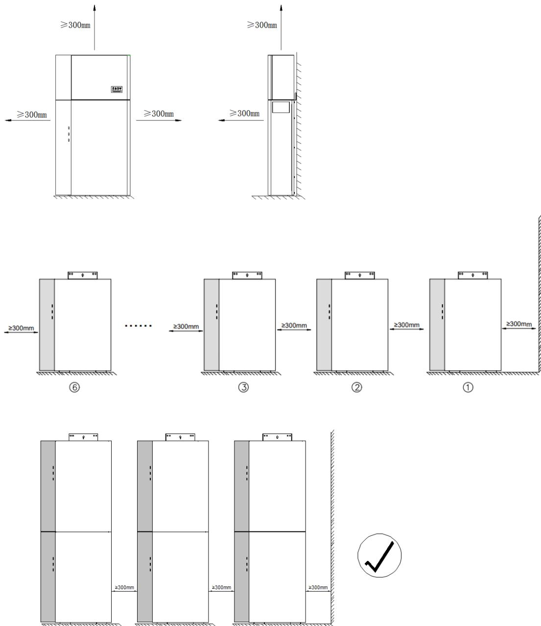
Recommended clearances for series batteries
