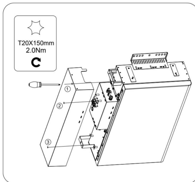
Mount the left cable cover of the battery SMILE-G3-BAT-10.1P, then install the right breaker cover, detailed steps are as follows:
