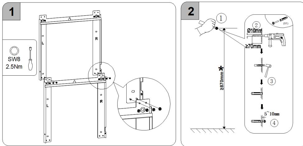
\*This recommended value "870mm" is for wall bracket location of the second battery seeing from the bottom up. Depends on the number of expansion batteries mounted later.
