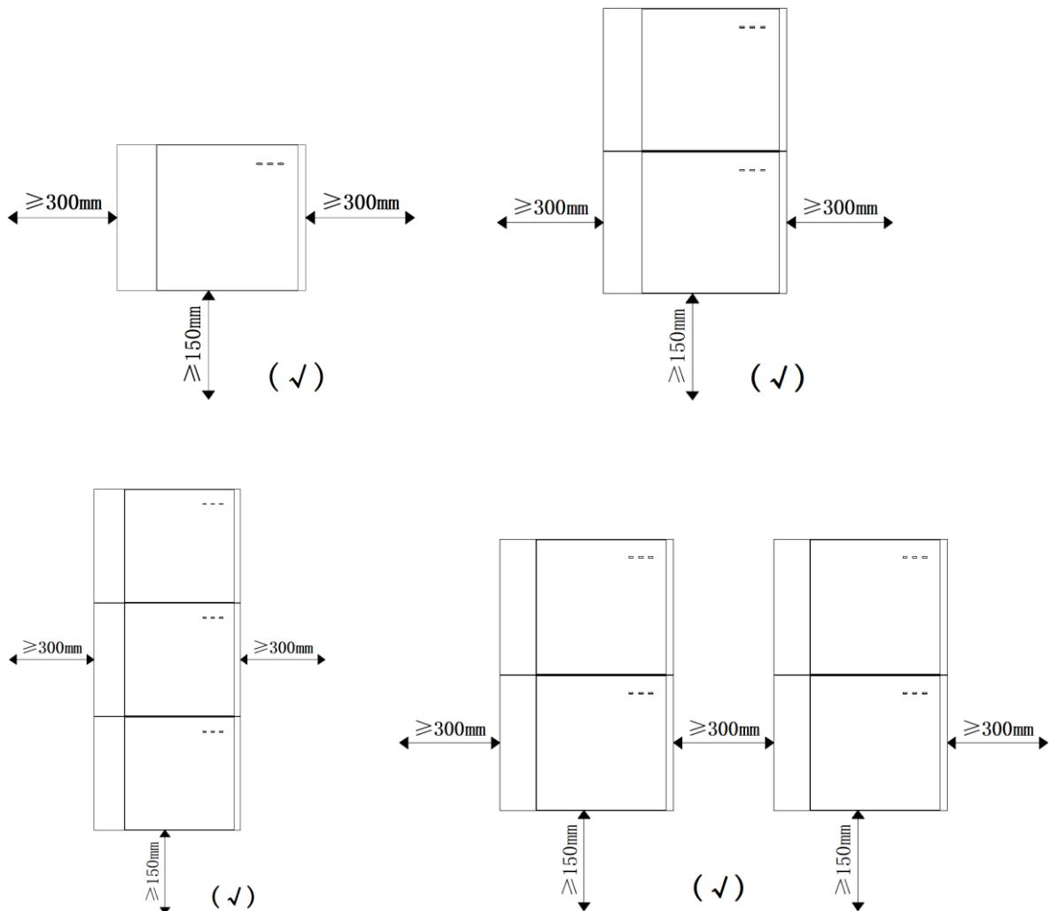
Local Standards may add additional clearance requirements, particularly regarding clearances between the Battery System and other Electrical Appliances.
